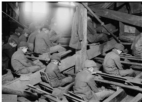
Breaker boys sort coal in an anthracite coal breaker near South Pittston, Pennsylvania, 1911.
